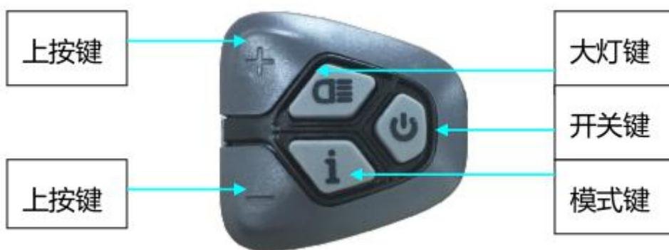
**5. 1. power switch:** press button for 2 seconds to open meter, press 3 seconds to down meter. If you do not operation meter in 5 minutes it can be closed.
