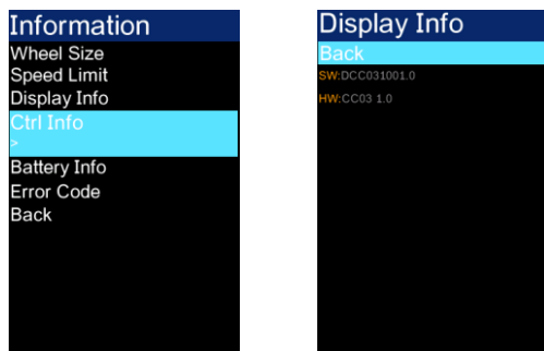
Check controller’s information
